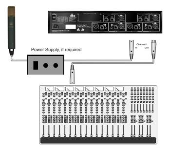
Figure 1: Connecting a Mic to a console.
