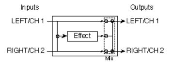
• Mono-in/stereo-out. These effects have a single mono input and two outputs.
