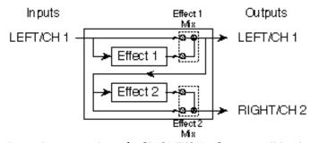
*Note:* If Cascade mode is turned on, the [RIGHT/CH. 2] input will be disabled for all Dual Mono Configurations. This is because the channel 2 effect is being fed the output of the channel 1 effect.
