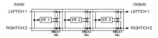
In the case of Multi Chain Configurations, the "Mix" parameter of each effect determines what the following effect receives at its input(s). *Example*: It is possible to use the "Delay->Room" Configuration (where effect 1 is a mono delay and effect 2 is a reverb), and have only the dry, uneffected signal going to the second effect; this is done by setting the first effect's Mix parameter to 000% (this means none of its output can be heard nor is sent to the second effect in the chain).
