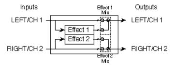
These effects can be chained using a special feature called Cascade mode. Cascade mode only affects Dual Mono Configurations, and routes the output of the channel 1 effect into the input of the channel 2 effect. The Cascade function can be turned on and off from page 2 in Utility mode (see Chapter 5). In this case, the Left/Ch. 1 output provides only the channel 1 effect's output, while the Right/Ch. 2 output provides the output of channel 1's effect routed through channel 2's effect.
