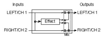
• Stereo-in/stereo-out. These effects have two inputs and two outputs.
