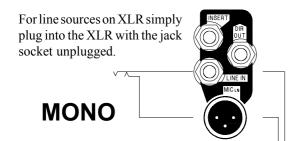
Plug in a microphone or line level source. Use balanced cables where possible to prevent interference pickup on long cable runs. Unbalanced sources may be connected by linking signal cold to ground (XLR pin 3 to pin 1, jack ring to sleeve) at the connector.
