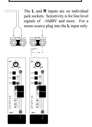
2 Stereo return inputs are provided to return the effects ('wet') signal, usually from a stereo device, to the mix. These are normally routed to the main **L-R** mix but may be returned to the corresponding pairs of subgroups for group effects (1-2 or 3-4).
