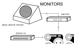
**AUX 1-4** balanced outputs feed foldback monitors with graphic EQ on **INSERT** to tune out acoustic resonances or to minimise feedback. **AFL** lets you check the output signal after the insert and master level control.
